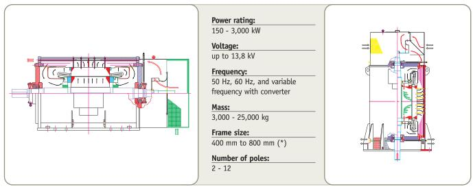
The following table shows typical values per size range for the series ET machines in 2 - 4 - 6 pole configurations. For further details please contact our Sales Office (See address below)
